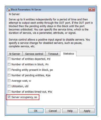
Selecting **Server occupancy**, **so** adds a signal output port labeled **so** to the block.
